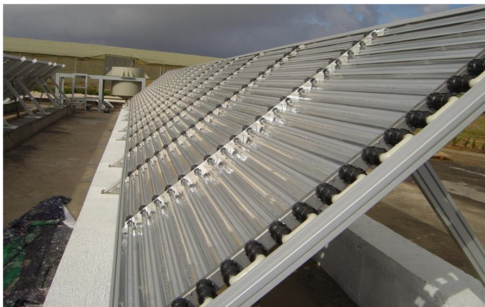
Fig. 3. CPC basic design and pilot plant.
