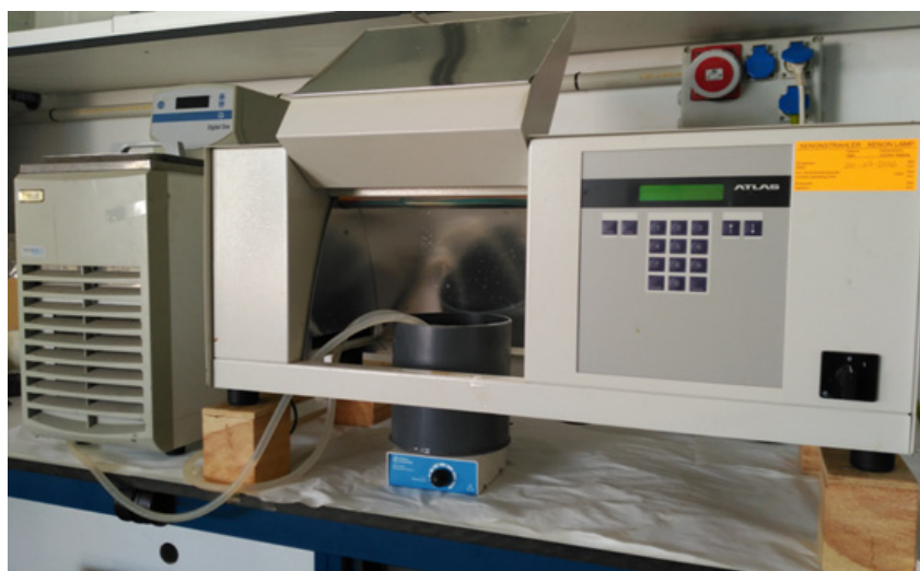
Fig. 9. SunTest CPS+ solar box with stirred tank reactor.
